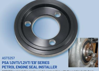
AST5257 seal installer can be used in conjunction with the existing bolts from the crankshaft pulley to drive the crankshaft seal to its final position within the engine casing. The seal is installed to a final position that is below the surface of the engine casing – standard installation adaptors will not install the seal to the correct position in the engine casing.
